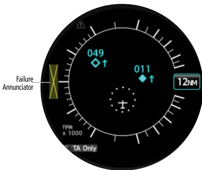
Vertical Speed Failure Annunciations
