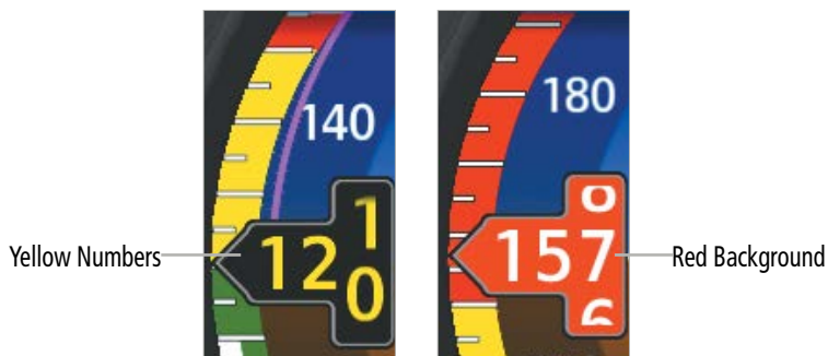
Airspeed Indicator (Approaching and Exceeding V NE )
